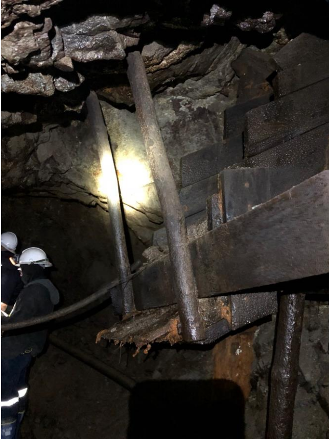
Photo 2: Box chute through which ore is released from a stope, a common practice in old mines.
